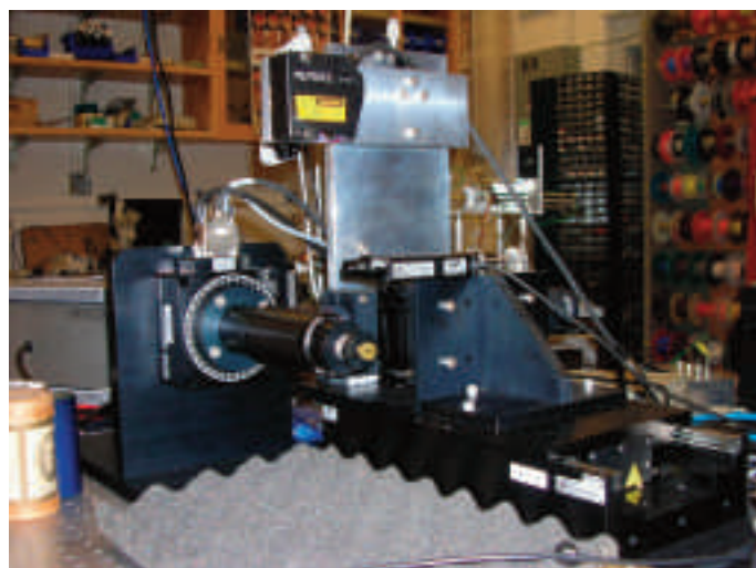
Figure 6: The 3D scanning hardware in place. Cylinder is in foreground. Laser sensor is above.
