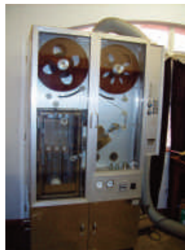
3. The ultrasonic cleaning machine - is not working. © National Archives of Zimbabwe
