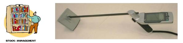
The components necessary for inventory management consist of a Reader and a Wand with an IPAQ (hand-held personal digital assistant) at the end. The Reader weighs only 607 grams (1.34 lbs) and the Wand 435 grams (0.96 lbs), making the weight of the entire unit approximately one kilogram. A shelf can be inventoried in a matter of a few minutes as the units can read up to 20 tags a second. The system allows for two different methods for taking inventory.
